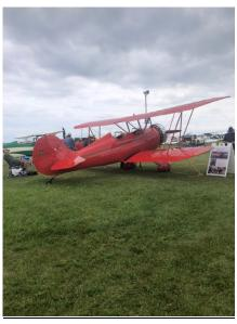
BUHL BULL PUP I have seen a few of these over the years usually hanging in the back of someone's hangar because the little three cylinder engine had died or was totally unreliable. There was a perfectly restored one with the three cylinder Szekely 45 hp engine. Originally it was designed by Etienne Dormoy, same guy as the Dormoy Bathtub. This particular plane was in perfect shape and didn't have all the dings and dents that every other one I had seen usually have.
